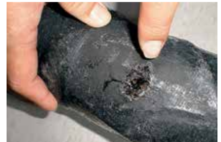
➤ Cable faults on paper-insulated mass-impregnated cable
