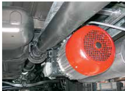
➤ Example of a synchronous generator, underfloor
