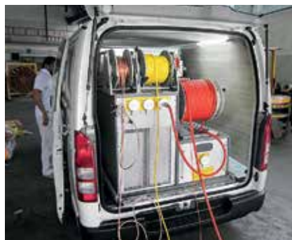
➤ Cable test vans of all sizes are equipped by BAUR.
