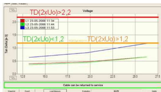
TD graph: Cable in good condition, <1.2 \cdot 10^{-2} @ 2 U_0 , IEEE
