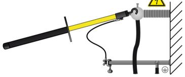
4. Immediately after earthing, connect the earthing and short-circuit equipment to the test object.
